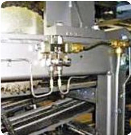
*Stainless steel SL-32 grease injectors are used here to prevent corrosion from daily "wash-down" maintenance practices at this food plant.*
