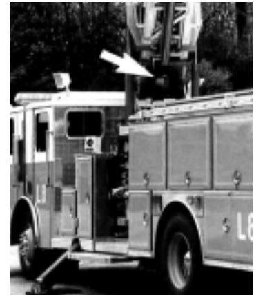
ON THE COVER: Typical Cable-Master® reel providing power to a tool at the end of a telescoping arm.
