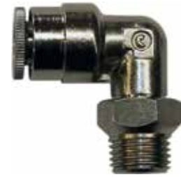
Elbow 90° Push-In Type With Knurled Collar for Plastic Tube
